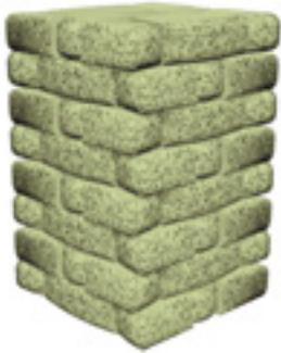
To build a 30-inch column, split two medium wall units in half. Stack column units in a rotating pattern for each course. Glue each course of units with a concrete adhesive. Round the split ends with a hammer and chisel. For more information about Highland Stone retaining wall products, see page 14.
