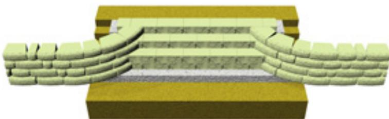
*Drainage Tip: Drain pipe can be placed behind the lowest step units at grade or behind each wall adjacent to the steps.*
