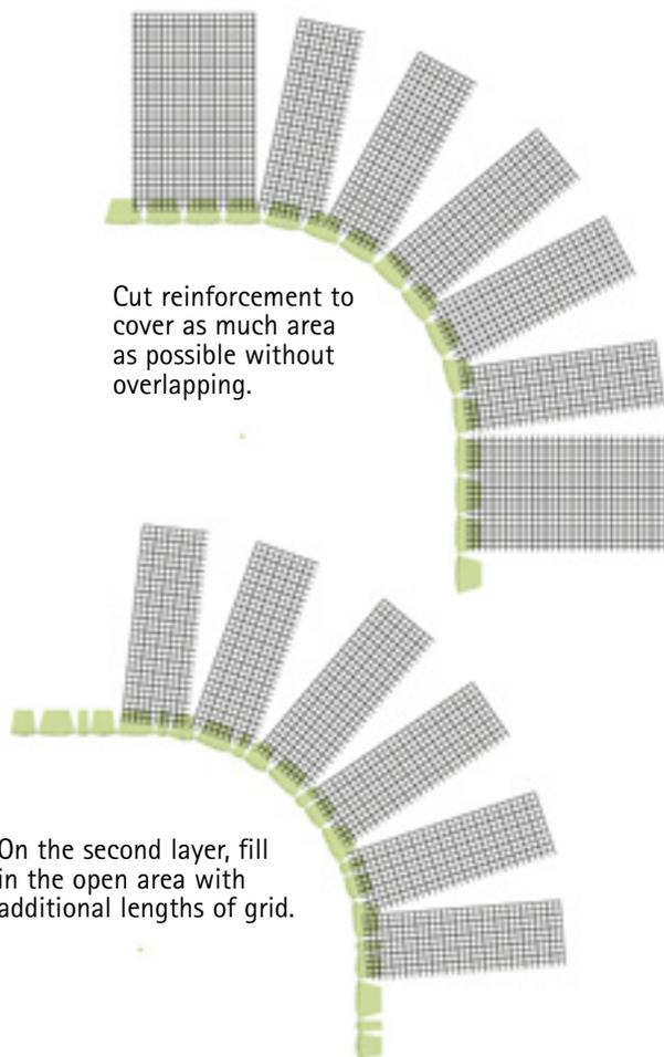
Cut reinforcement to cover as much area as possible without overlapping.
