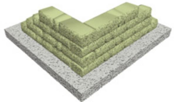
To create a 90° corner in a straight wall, make a third side to a large unit by splitting it to the appropriate dimension. Use only large units to assure connecting units are on bond. Alternate the direction the units face with each course. Round the split ends with a hammer and chisel. Glue all corner courses with a concrete adhesive.
