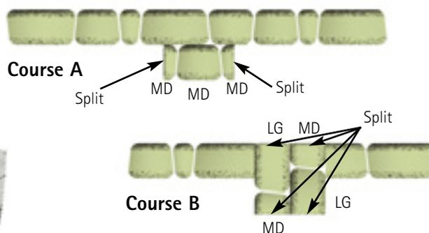
**SMALL PILASTER AT END OF WALL**
