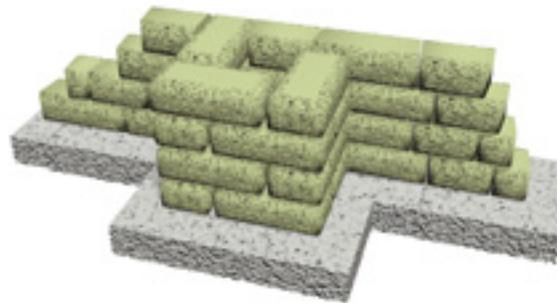
**PILASTER AT END OF WALL**
