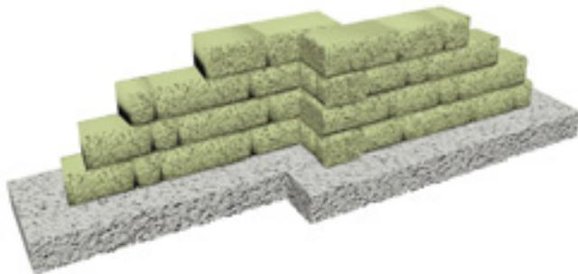
Jogs are used to break up straight lines and add stability to walls. Split units as needed. Use hammer and chisel to round split faces. Glue all courses of jog with a concrete adhesive.
